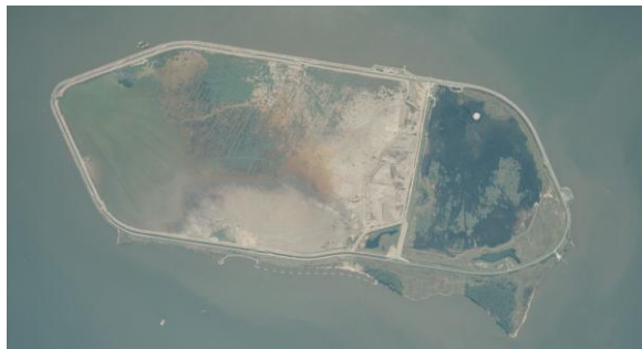
An aerial view shows the containment dike, which creates a secure settling basin for dredged material.
