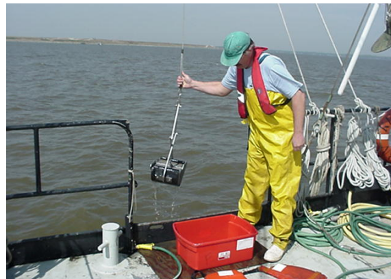
A small dredge collects samples of sediment and organisms from the floor of the Bay.
