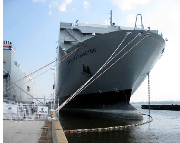
The Maritime Environmental Resource Center uses the M/V Cape Washington, located in the Port of Baltimore, to test ballast water treatment systems.
