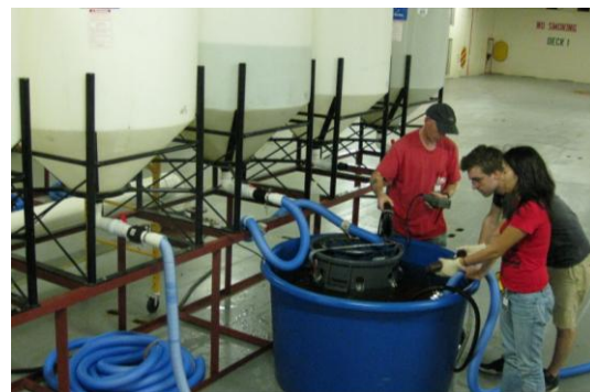
A testing team collects and analyzes water samples to determine how well shipboard treatment systems remove or kill non-native organisms found in the ballast water of ships.
